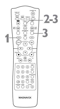
Press DISPLAY repeatedly or press RETURN to remove the display.
